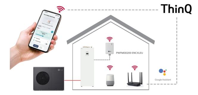
PWFMDD200 (LG Wi-Fi Modem) / PWYREW000 (10 m extension connect cable in between THERMA V indoor and LG Wi-Fi Modem) could be required depending on
